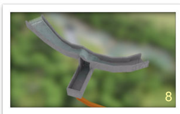
DEBRIS BYPASSES THE TURBINE - 8
